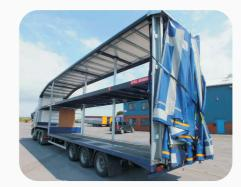
Wrap around curtains give a full clear side aperture. The design is ideal for pallet hub operation.
