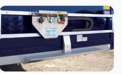
Developed to aid safety, MAVIS (Montracon articulated vehicle interconnecting system) can be slid to either side of the trailer to facilitate un/coupling and eliminating the need for the driver to climb onto the chassis between the cab and trailer.
