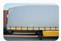
A roof line that cants at the front promotes attached air flow along the roof to improve the high roof trailer's aerodynamic envelope and improve fuel economy by up to 10%.
