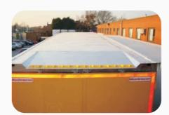
To boost fuel economy on a standard height straight frame curtainsider a fuel saving cant roof and vortex generators at the rear combine both to improve attached air flow and to channel the flow into the base drag area immediately behind the trailer.
