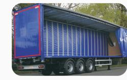
For a clear loading aperture Montracon offers two postless variants with either a straight or tapered cant rail to meet operator requirements.
