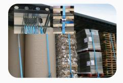
Montracon's Retractostrap promises to improve loading safety, load security and vehicle turnaround times. Handled from ground level, when loading, ratchet linked load retention straps are drawn along wires - on either side or down the middle of a trailer - over the load to the position required, the suspended strap then being easily retrieved and pulled down to couple with a strap/tensioner secured to a floor mounted lashing ring or drop down cleat in the side rave.
