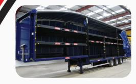
For maximum cubic capacity, Montracon offers the double decker on either a straight or step frame at overall trailer heights up to 4.8m. Apart from the movable/ratchet deck version shown, Montracon offers fixed, swivel and butterfly options.
