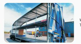
Wrap around curtains give a full clear side aperture. The design is ideal for pallet hub operation.
