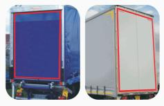
The choice of barn, flush and roller shutter rear doors. Barn doors feature robust, large diameter lock rods; flush doors are offered for better livery presentation; and shutters, including a wide lathe option, are offered for easier dock loading/unloading.
