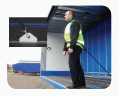
As its name implies, Montracon's Fallcheck checks the operator's movement at the side/rear raves while allowing free movement along and across a trailer bed.
