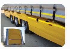
To further improve aerodynamic efficiency and fuel economy, the purpose designed front headboard aids attached air flow onto the trailer from the tractor's cab mounted deflector and side skirts minimise air turbulence along and under the trailer.
