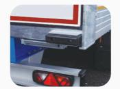
Carefully positioned reinforced buffers 29mm vertically laminated hardwood minimise the risk of damage when reversing up to a loading bay, for
