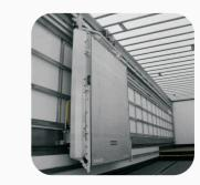
Internally installed lift, with fore/aft movement to ease loading and unloading capability.
