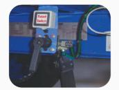
To ease loading/unloading, the trailer deck is easily raised or lowered at the rear to match dock height. An automatic trip restores the deck to example. normal running height on departure.
