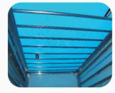
With an aluminium skin as standard. Montracon offer a GRP translucent roof or for loads that are susceptible to heat or moisture then a 30mm insulated roof is also available.
