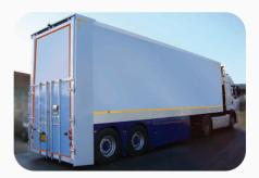
Rear door/tail lift arrangement designed to meet retail delivery requirement.
