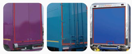
Vans can be fitted with either flush, barn or roller shutter doors at the rear, with a further option of having flush doors incorporated along either or both sides. Barn doors feature large, robust, large diameter lock rods, flush doors are offered for better presentation of livery and shutters, including wide lathe shutters, are offered for quicker dock loading/unloading to speed multi-drop operations.
