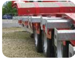
Outriggers extending deck by max 600mm
