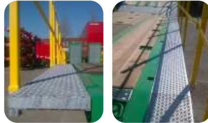
Gripped walkways allow the driver to maintain safe access along the deck even when the load takes up the full width of the trailer bed.
