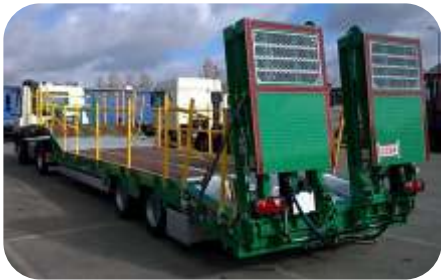
Tandem axle step-frame machinery carriers can be more manoeuvrable than rigid beavertail trucks when it comes to small local plant deliveries.
