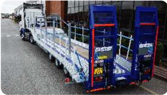
Pull out Hi-Vis handrails and driver fall arrest protection.
