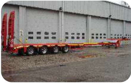
The four axle centre spine extendable machinery carrier with rear steer axle(s).
