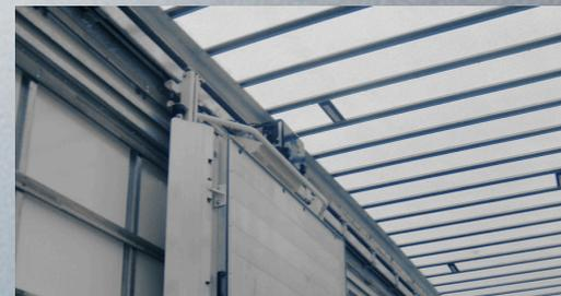
Internally installed lift, with fore/aft movement to ease loading and unloading capability.
