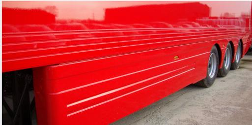
Side skirts promote attached air flow along the trailer sides. Vortex generators direct attached air flow to the base drag area immediately behind the trailer to reduce drag.
