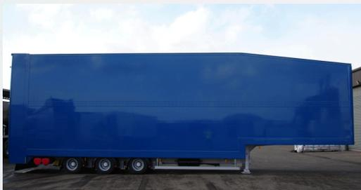
A sloped roof design promotes an attached air flow to improve the aerodynamic envelope & the fuel economy achieved with the max height trailer. Savings as high as 10% have been reported for overnight motorway trunking operations.
