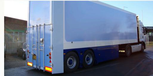
Rear door/tail lift arrangement designed to meet specific retail delivery requirements.
