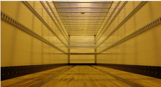
'High gloss' finish inside and out helps to maintain a clean, neat appearance, with an ample kick strip providing scuff protection during loading/unloading. Load restraint rails are side panel mounted.
