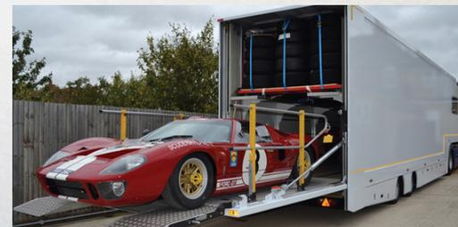
Engineered to accommodate racing cars and crew, yet be low enough to access the pits via tunnels under the race track.
