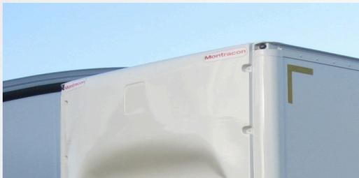
A purpose designed front headboard promotes efficient air flow around the trailer from the tractor units cab mounted deflector.
