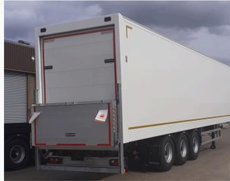
Our vans can be fitted with flush, barn or roller shutter doors at the rear, with a further option of having flush doors incorporated along either or both sides. Barn doors feature robust, large diameter lock rods, flush doors are offered for better presentation of livery, and shutters, including wide lathe shutters, are offered for quicker dock loading/unloading to speed multi-drop operations.
